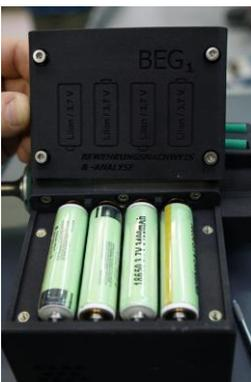
When all the batteries have been fitted in place, close the cover with the four screws.
