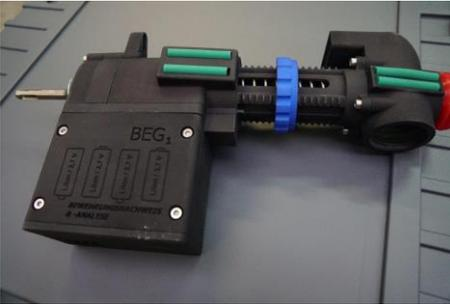
Undo the four screws on the cover of the battery compartment using the hex. socket screwdriver supplied.
