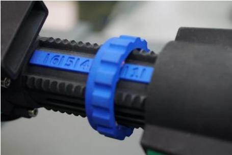
Set the stop ring to the desired incremental depth position and lock by turning to the right.
