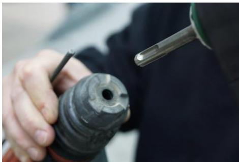
Insert the BEG<sub>1</sub> into a standard battery or mains powered hammer drill with an SDS-Plus chuck.
