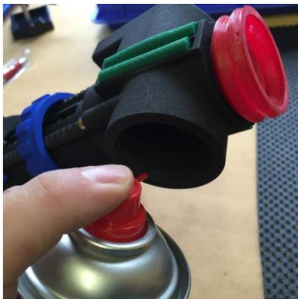
Clean the drilling head and the equipment with compressed air spray after each sample taking.
