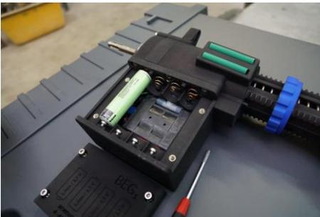
Place the charged batteries as illustrated on the cover noting the +/- labelling.
