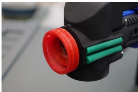
Press the seal together with the fingers and pull off to the front. Similarly press the new seal together and put it in place.
