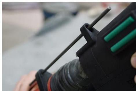
Secure the anti-twist device using the depth stop on the hammer drill.
