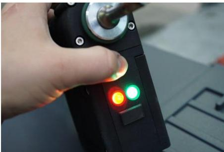
If the equipment is ready for operation, the red and green LEDs light up, the sound of the pump can be heard and air flows from the drill.
